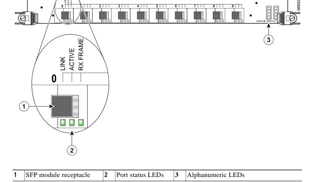
Table 6 summarizes the optics and connectors used by the 10-Port 1-Gigabit Ethernet line card.
